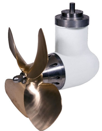
Four Blade Kaplan Style Propeller
